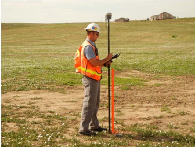
Figure 2: Ground positioning error increases with pole tilt
