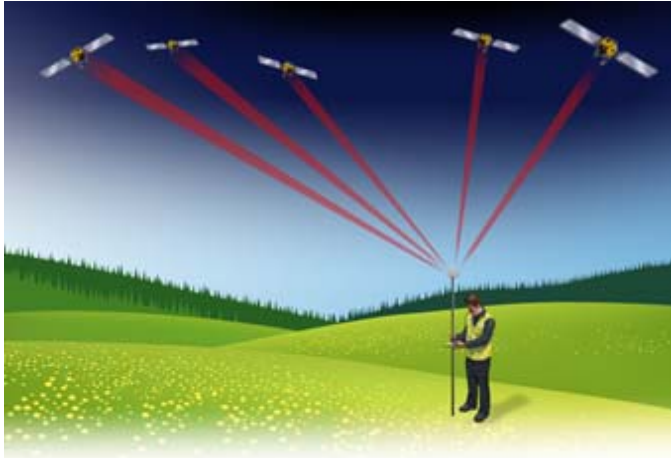
Figure 1. Trilateration of satellite ranges to estimate an autonomous receiver's position
