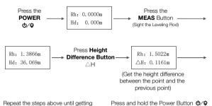
**ATTENTION:** To store the results of this measuring mode, press the Store Button **REC** ▲. To exported data to computer, install software that was included with instrument when purchased.
