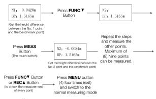
**NOTICE:** Press  $\Delta H$  key to switch between the display of leveling rod reading of the benchmark point and the display of the sighting distance of the current measuring point.
